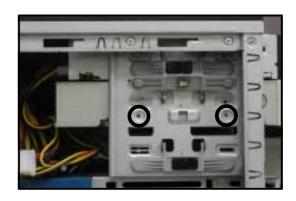
8. Pull down the bar lock and insert the lock pegs to the drive/bay holes, then push the drive lock to the right to secure the drive.
